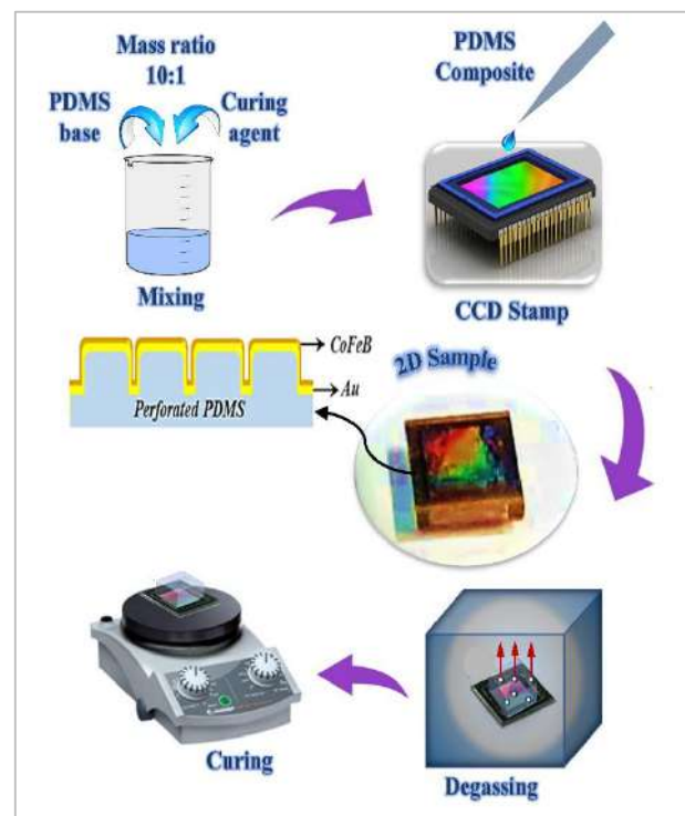
Figure 1: A schematic array of the fabrication process of the CoFeB perforated microstructure.
