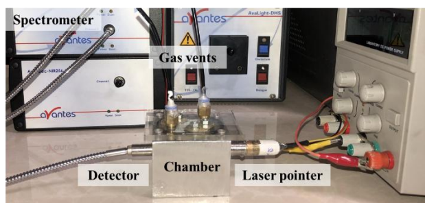
Fig. 2: Optical setup for PL measurements
