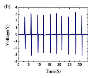
**Figure 2.** (a) Frequency response of GPG-based acoustic device: variation of sound pressure level (SPL) as a function of frequency within a broad region (1~3000Hz). (b) Output voltage of the GPG-based nanogenerator as a function of time.
