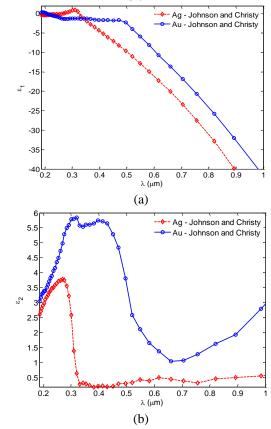
Figure 2: (a) Real and (b) imaginary parts of the relative permittivity of gold and silver [15].
