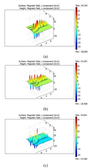
Figure 3: 3D plot of the z component of magnetic field [A/m] of three operating states of the optical OR gate, a) 0-1 b) 1-0 c) 1-1.
