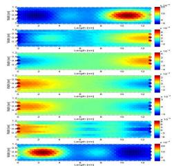
Fig. 4: Local photocurrent across the photodetector with Au-Ti leads under biasing conditions of  $V_{\rm DS}{=}0$  and  $V_{\rm GS}{=}$  (a) -80 mV, , (b) -40 mV, (c) -20 mV, (d) 0, (e) 20 mV, (f) 40 mV and (g) 80 mV. Color bars indicate the local currents in units of  $\mu A$ .
