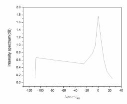
**Fig. 2.** CS intensity spectrum in nonlinear gain; Parameters are  $\left|E_{0}\right|^{2}=0.58$ ,  $\left|E_{m}\right|^{2}=0.05$  and  $\upsilon_{RO}=110GHz$ .
