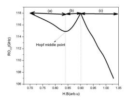
**Fig. 1.** relaxation oscillation frequencies as a function of laser holding beam in CS for nonlinear gain 20% above threshold. (a) and (b) Hopf bifurcation and (c) locking area zones.
