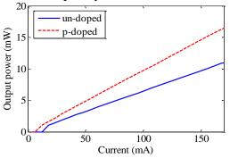
Figure 1- L-I characteristics of un-doped and p-doped QD lasers at temperature T=300K.
