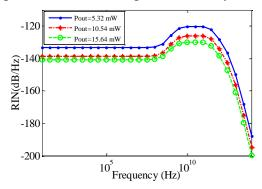
Figure 3- RIN value of p-doped QD laser with doping concentration of Na= $5\times10^{16}(cm^{-3})$  at three current density of  $J_1$ =6,  $J_2$ =12 and  $J_3$ =18 (kA/cm<sup>2</sup>)
