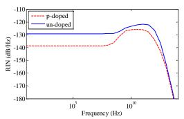
Figure 2- RIN in p-doped with doping concentration of  $N_a$ =5×10<sup>16</sup>(cm<sup>-3</sup>) and un-doped QD lasers at I=12 (mA)
