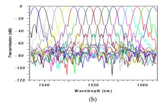
Figure 2: output spectra of a 16 channel AWG (a) device based on primary designed parameters and b) flatten response by applying new changes to the star couplers.
