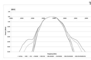
Figure 4: Filtering effect of different components on 100 Gb/s signal
