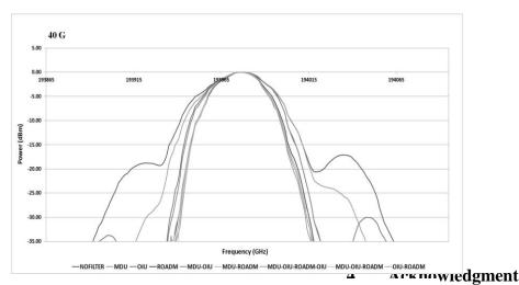
Figure 3: Filtering effect of different components on 40 Gb/s signal
