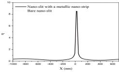
Fig. 2. Transmission efficiency η of nano-slit on x direction, without the nano-strip (dashed line) and with the metallic nano-strip (solid line).
