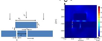
Fig. 3. (a) Schematic of the simulated structure consists of two nano-slits with distance d. (b) distribution of the magnetic field Hy with  $W_p$ =1  $\mu$ m and thickness of Hp=300nm, G=40nm and t=44nm and g=10 nm.
