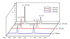
Fig. 4. Transmission efficiency of the two nano-slit structure for different size of the lateral nano-slit (g).
