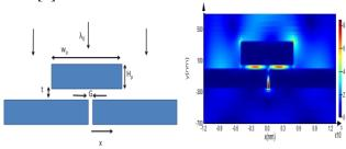
Fig. 1. (a) Schematic of the simulated structure and geometric parameters. Both the film and the nano-strip are made of silver ( $\varepsilon$ Ag= -48.8+3.16i [19]). (b) Distribution of the magnetic field Hy with  $W_p$ =1  $\mu$ m and thickness of Hp=300nm, G=40nm and t=44nm. The X arrow in fig (a) shows the beginning of the X axis in fig (b).
