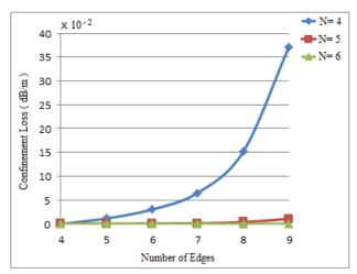
Fig.4 Plots of C.L against the number of edges for  $d/\Lambda = 0.5$  at  $\lambda = 1.55 \mu m$
