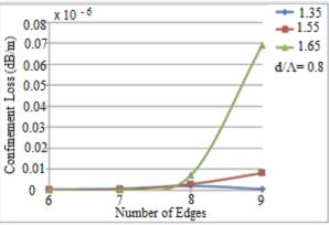
Fig.2 Plots of C.L as a function of the number of edges when N=4 for various  $d/\Lambda$
