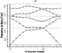
Figure 2: Dispersion curve for PC with R = 130 nm and a = 380 nm excited by light with (a) TE polarization and (b)TM polarization.
