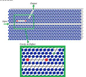
Figure 3: the resonant cavity with its defects.
