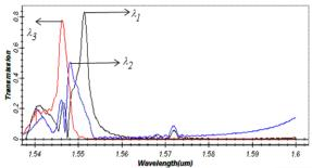
Figuer 6: Representation of the demultiplexer output channels at  $\lambda 1$ ,  $\lambda 2$  and  $\lambda 3$  wavelengths.
