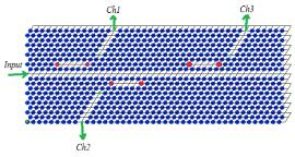
Figuer5: Schematic design of seven channel demultiplexer based on photonic crystal waveguide.
