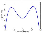
Figure 3: Dispersion profile of the optimum waveguide
