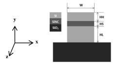
Figure 1: Structure of the waveguide
