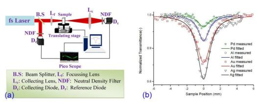
Figure 2. Open-aperture Z-scan setup (a) and Z-scan data for different samples (b).
