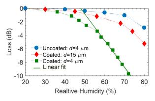
Fig. 5: Comparison of the sensor response for an uncoated TMMF (circles) with those of similar TMMFs coated with silica gel (diamonds:  $l \approx 8$  mm,  $d\approx 15$  µm). The lengths and diameters of the waist regions of both sensors were  $l\approx 9$  mm and  $d\approx 4$  µm.
