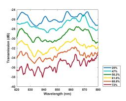
Fig. 4: Transmission spectra through the sensor with l = 9 mm and d = 4 µm for different RH%
