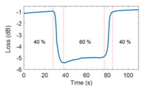
Fig. 6: Time characteristic for the sensor with the l=9 mm and d=4  $\mu$ m
