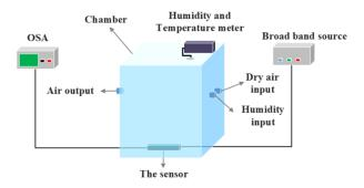
Fig. 3: Schematic of the characterization setup.
