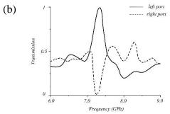
Fig. 3: (a) The electric field profile at f=7.25 GHz shows that propagation of the electromagnetic field is only allowed to the left in the waveguide. The inset shows the direction of the propagating light can change by the direction of the applied magnetic field. (b) The transmission spectrum of the waveguide shows that at f=7.25 GHz all the energy is propagated to the left port and zero energy is received at the right port.
