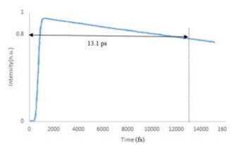
Fig. 3: Integration time of the optimized ring resonator.
