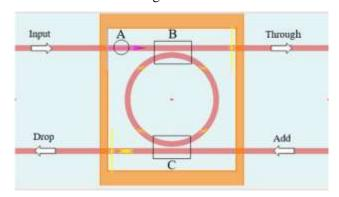
Fig. 1: Ring resonator simulation with a radius of 3 micron.
