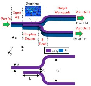
Fig. 1: The structure of the proposed PBS.
