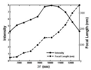
**Fig 2**: Intensity and focal length of PNJ created with circular cylinder versus radius of cylinder.
