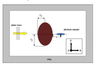
**Fig.1**: Schematic diagram of an elliptical dielectric cylinder for photonic nanojet.
