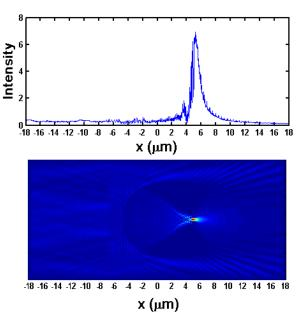
**Fig 3**: Intensity distribution of circular PNJ with diameter of 10125 *nm*.
