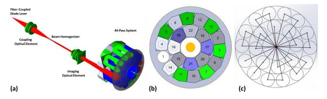
Figure 1.a) Schematic of the designed pumping optical system. b) The sequence of used flat mirrors. c) Propagation of pump beam in 44-pass system
