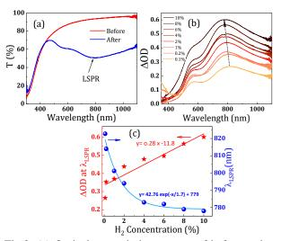
Fig.3: (a) Optical transmission spectra of before and after exposure 0.1% hydrogen exposure at 150 °C operating temperature (b) Typical LSPR optical  $\Delta$ OD spectra of Pd/MoO<sub>3</sub> film at 0.1-10% hydrogen exposure and (c)  $\Delta$ OD at  $\lambda$ <sub>max</sub> and  $\lambda$ <sub>LSPR</sub> as a function of hydrogen exposure
