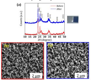
Fig.2: (a) XRD patterns of Pd/MoO<sub>3</sub> thin films before and after hydrogen exposure, the SEM images of thin films before (*b*) and after hydrogen exposure(*c*).
