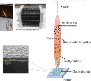
Fig.1: Schematic representation of oxyhydrogen generator and flame, flame synthesis of MoO<sub>3</sub> films and a cross-section FESEM image of produced films.
