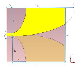
Fig. 1: Geometry of the proposed antenna
