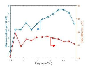
Fig. 3: Simulated realized gain and total efficiency of the proposed antenna.
