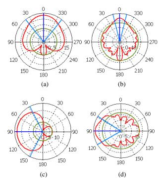
Fig. 4: Far field pattern of the E field in the XY plane ( $\theta = 90^{\circ}$ ) at (a) 0.5 THz (b) 2.5 THz and in the XZ plane ( $\varphi = 0^{\circ}$ ) at (c) 0.5 THz and (d) 2.5 THz
