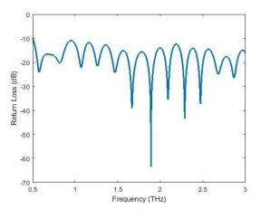
Fig. 2: Return loss of the proposed antenna.
