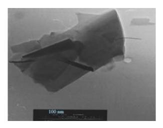
Figure 1: TEM image of graphene synthesized by laser
