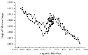
Figure 4: magnetic curve of hybrided graphene.
