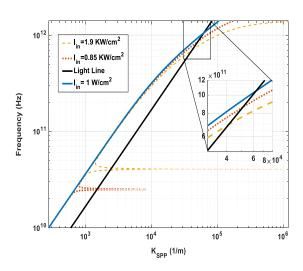
Fig. 4: Dispersion curves for three different input intensities.
