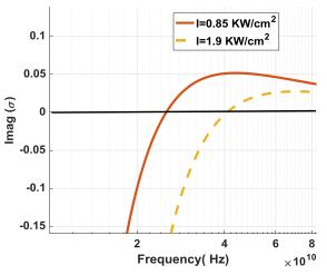
Fig. 6: Imaginary part of conductivity versus frequency.
