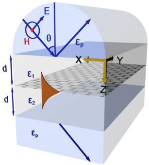
Fig. 1: Configuration of Kretschmann-Raether structure [8].
