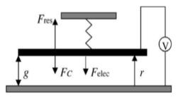
Fig. 1: (a) schematic of cantilever switch, (b) Onedimensional lumped model for the pull-in parameters estimation [2]-[7]
