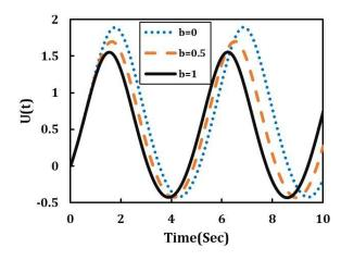
Fig. 3: Variation of pull-in gap with respect to time for three different values of b=0, b=0.5, b=1
