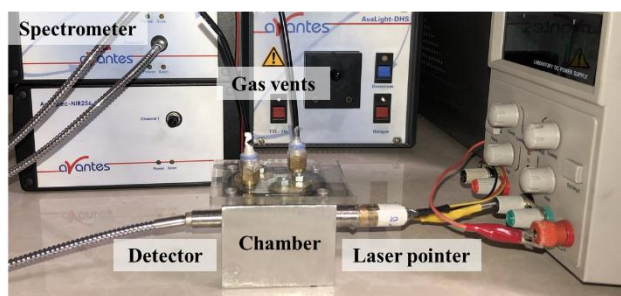
Fig. 2: Optical setup for PL measurements
