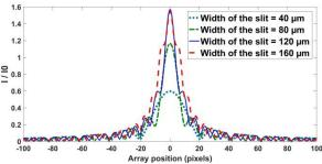
Fig. 3: The diffraction pattern with different aperture sizes at h = 8 mm.
