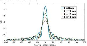
Fig. 5: The diffraction patterns of a slit with width =  $80\mu m$ , with respect to different h.
