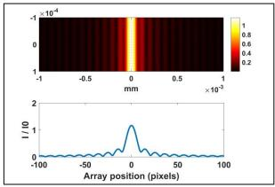
Fig. 4: The Fresnel diffraction model of Sun sensor with a slit aperture with width =  $80\mu$ m on the detector plane.
