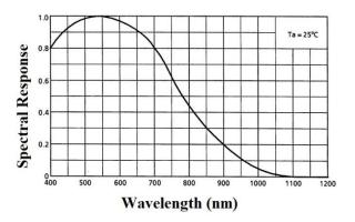
Fig. 2: Spectral response curve of the detector.
