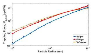
Fig. 2. Maximum Trapping force in the z direction versus particle radius with l = 3 nm.
