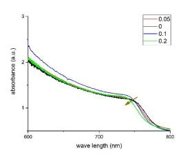
Figure 4 Visible spectra of the pure and mixed perovskite films.
