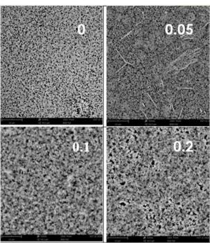
Figure 2 SEM images of the surface of the perovskite films comprising different concentrations of CsCl in the precursor solution (0, 0.05, 0.1, 0.2 molar).
