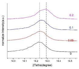
Figure 3 (a) XRD spectra of the perovskite films comprising different concentrations of CsCl in the precursor solution, and (b) a high resolution view of the (110) diffraction peak of the  $MA_{1-x}Cs_xPbI_3$  samples.
