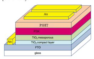
Figure 1 Schematic of the fabricated device structure.
