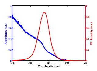
Figure 6: PL spectrum and absorption spectrum of FAPbBr<sub>3</sub>
