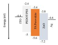
Figure 3: The energy level diagram of ITO/PEDOT: PSS/FAPbBr<sub>3</sub> perovskite/ZnO/Ag device.
