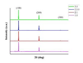
Figure 5: XRD patterns of FAPbBr<sub>3</sub> synthsized from precursors containing different ratios of FABr: PbBr<sub>2</sub>
