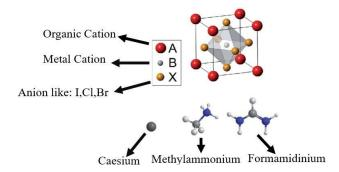
Figure 1: The crystalline structure of perovskite material.
