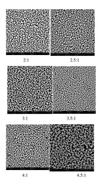
Figure 4: SEM images of the perovskite layers synthsized from precursors containing different ratios of FABr: PbBr<sub>2</sub>, (SEM images scale bar is 10μm).
