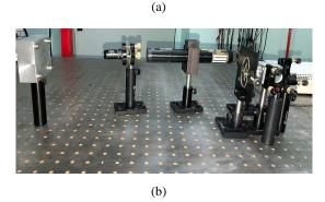
Fig. 2. (a) Schematic of proposed shearography setup: beam expander (BE), slit (S), beam splitter (BS), reference mirror (M1), tilt mirror (M2). (b) Realization of the setup.
