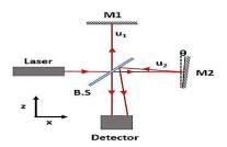
Fig. 1. Schematic of Michelson interferometer.
