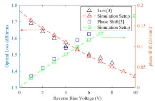
Figure 2. Optical loss and phase shift vs reverse bias voltage for [3] and this work simulation setup results.
