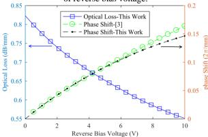
Figure 5. Optical loss and phase shift efficiencies vs reverse bias voltage, in the proposed modulator. The  $\pi$  radian phase shift is achieved in -9 V ( $V_{\pi}$ = -9 V).
