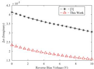
Figure 4. Refractive index imaginery part as a function of reverse bias voltage.
