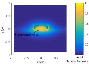
Figure 6. Phase shifter active area optical mode profile.
