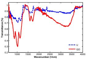
Figure 3: FTIR spectra of the prepared graphene sheets on  $SiO_2/Si$  substrate.
