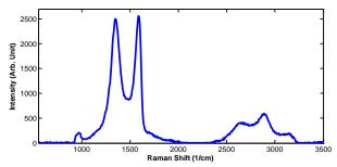
Figure 2: Raman spectroscopy of the prepared graphene sheets on SiO<sub>2</sub>/Si substrate.
